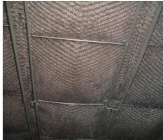
*In order to avoid droplets in off gas there is a mesh grid on absorber top*
