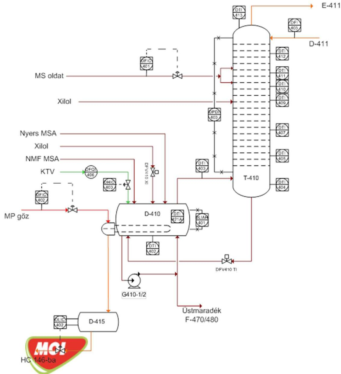
The distillation is not continuous but batch process and consists of several steps:
